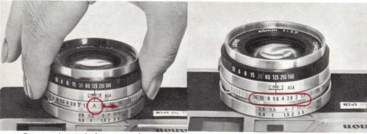
For manual control of aperture, release aperture ring from "A" position. The shutter speed and f/stop can be freely set for achieving specialized technical effects. With the Canonet G-III, special effects in high key or low key can be obtained in the same manner as with high-grade cameras.
